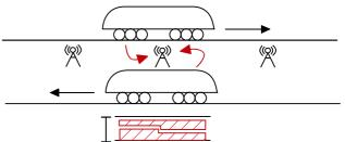
Probe feedback for data prioritisation allows these vehicles to prioritise critical traffic (such as control data and logs) whilst reducing non-essential traffic such as CCTV video feeds, or, in extreme cases, cutting the video feed entirely when reduced to low bandwidth auxiliary connections.
